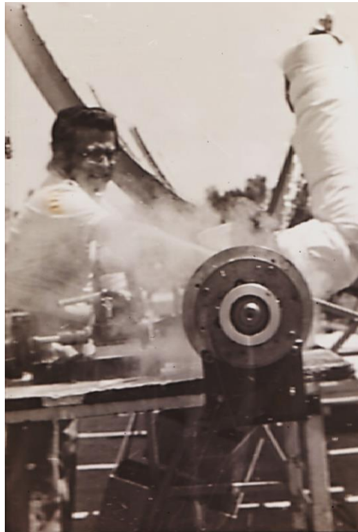
Figure 5.9 Rotary engine operating with solar generated steam
