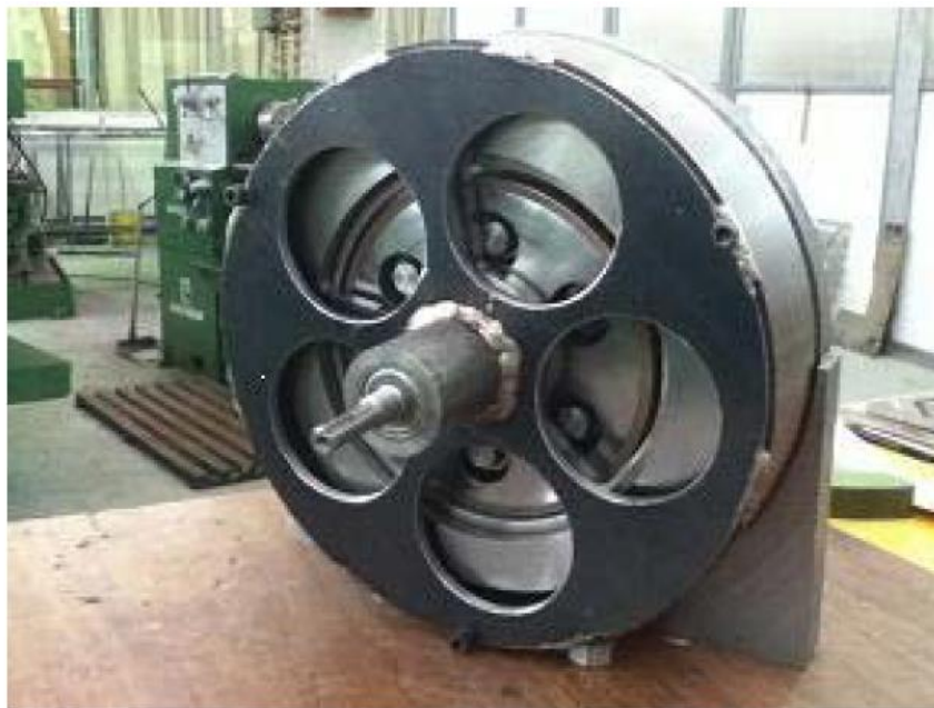
Figure 7.2 Cycloidal magnetic gear speed reducer prototype
