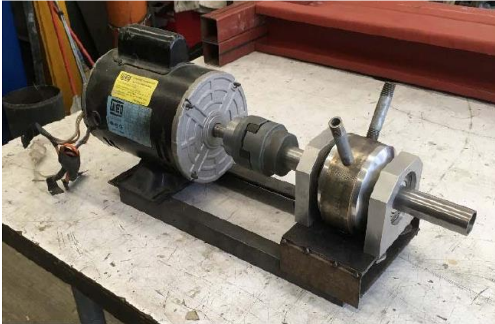
Figure 4.2 Resonant vane vacuum pump prototype
