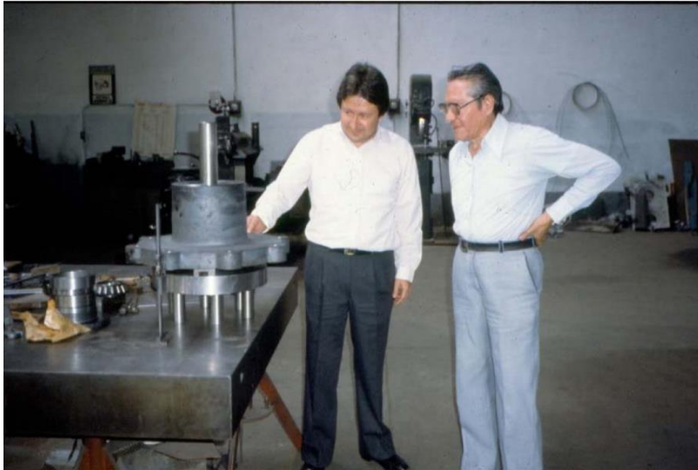
Fig. 1.3. Partially assembled pump for pumping molasses
